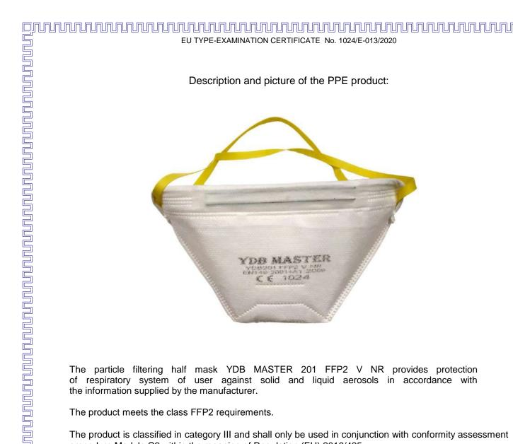
The particle filtering half mask YDB MASTER 201 FFP2 V NR provides protection of respiratory system of user against solid and liquid aerosols in accordance with the information supplied by the manufacturer.
